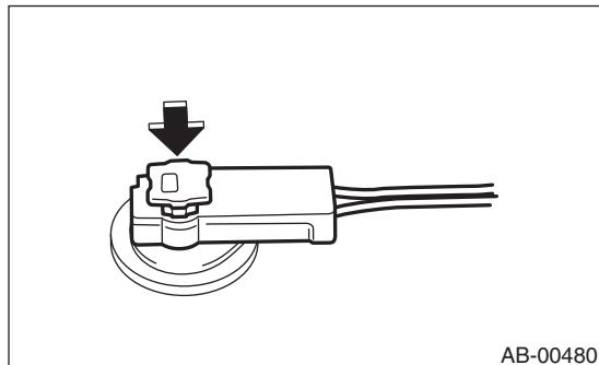
Connect the connector in the reverse order of disconnecting. At this time, be sure to insert until a clicking sound is heard.
