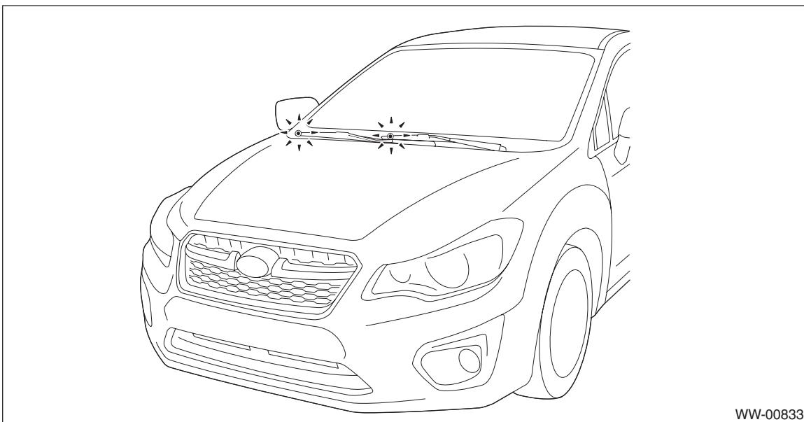
3) If the wiper blade is not aligned with the point mark, perform the removal and installation of the windshield wiper. <Ref. to WW-27, REMOVAL, Front Wiper Arm.>
