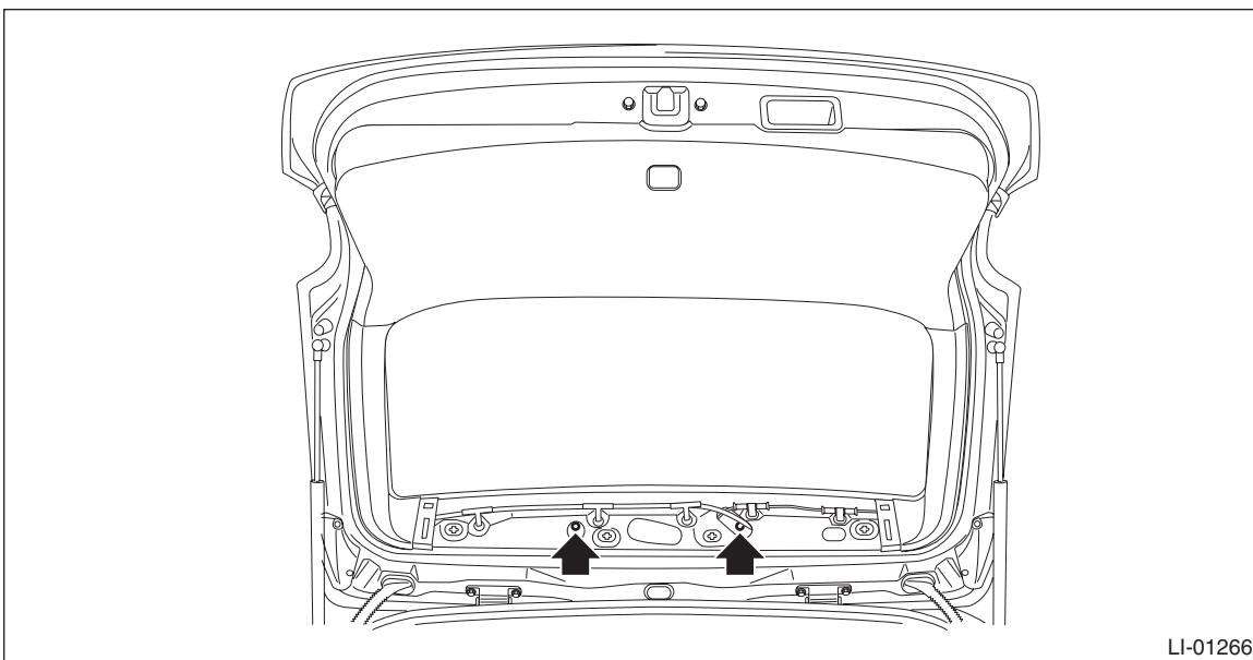
(2) From the inside of the rear gate, push the claws on both side of the light assembly - high-mounted to take it out toward vehicle rear.
