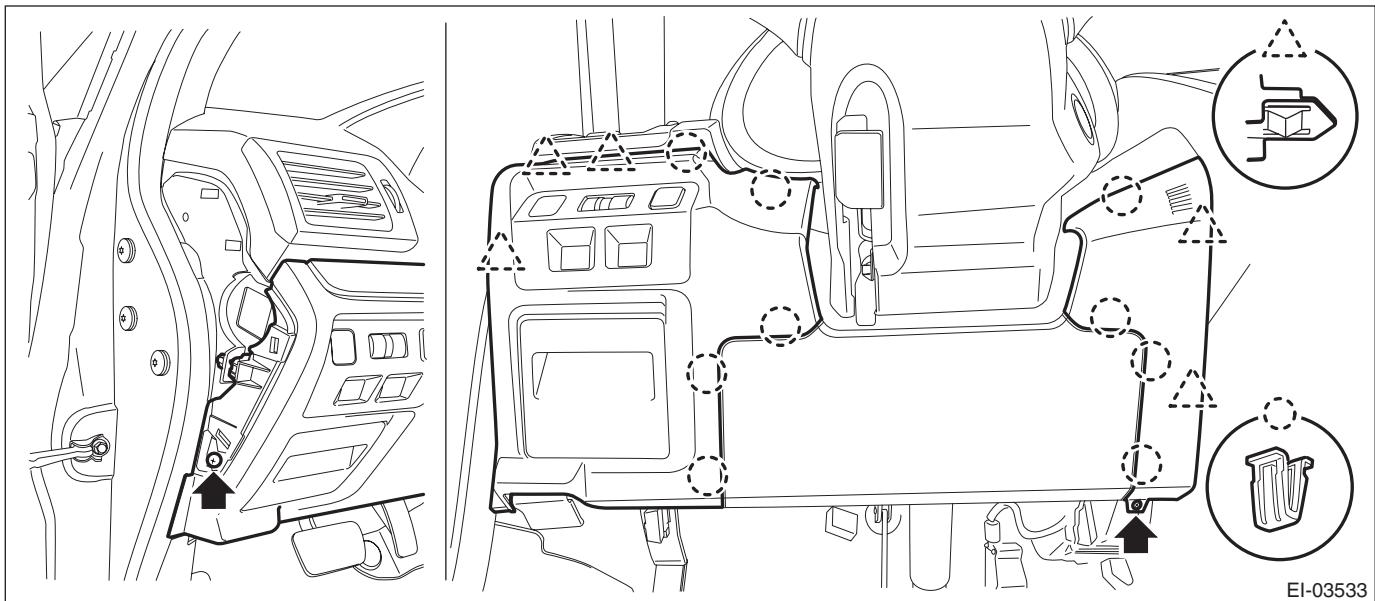
4) Remove the nuts to remove the knee airbag module and disconnect the harness connector. <Ref. to AB-33, KNEE AIRBAG MODULE, PROCEDURE, Airbag Connector.>
