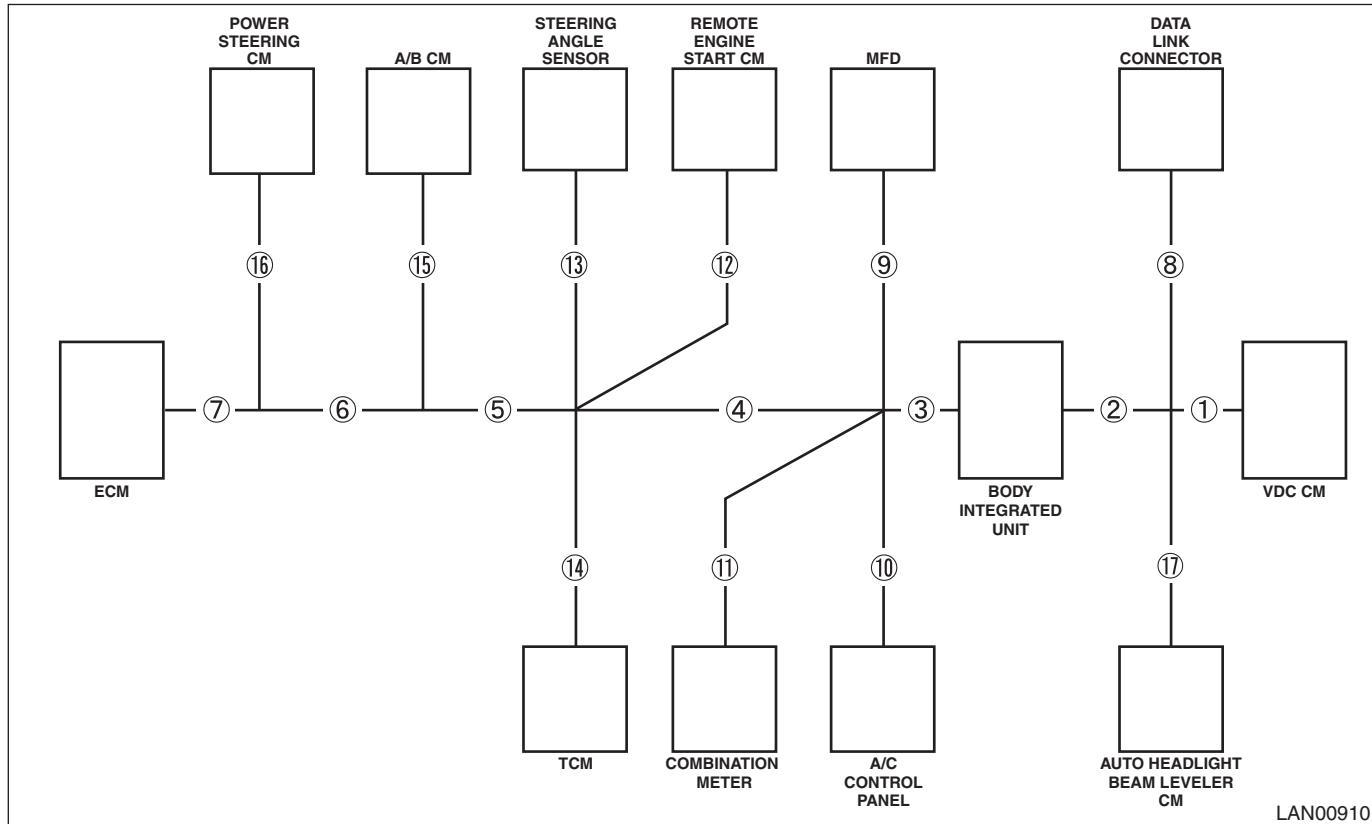
When ④ (main wiring harness between combination meter and steering angle sensor) is open
