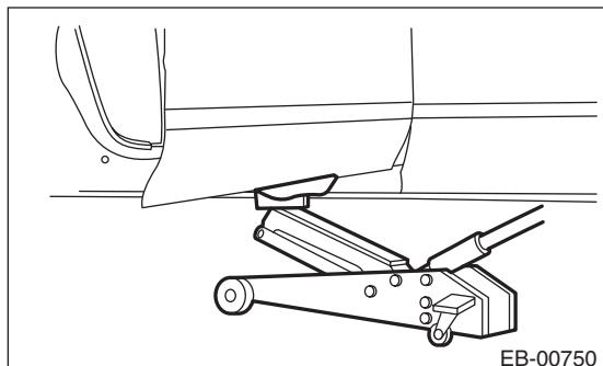
(1) Put a wooden block on a floor jack and place the jack under the panel assembly - rear door.
