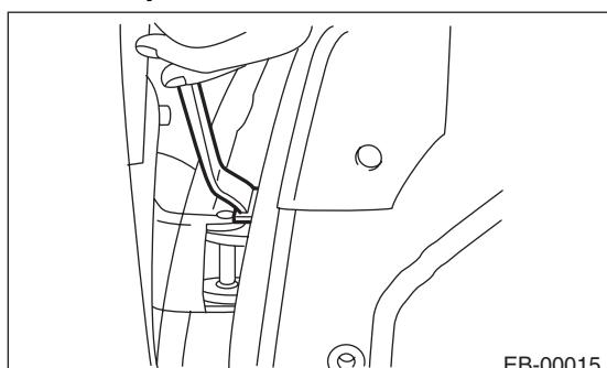
15) Remove the door hinge from vehicle. <Ref. to EB-36, REAR DOOR HINGE, REMOVAL, Rear Door.>
