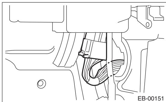
(2) Push in the claws to remove the grommet, and pull out the door harness connector.
