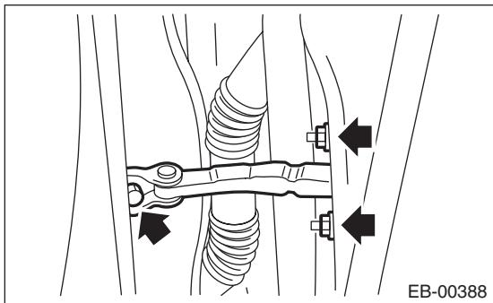
14) Release the claws, and then remove the cover side sill - front INN.
