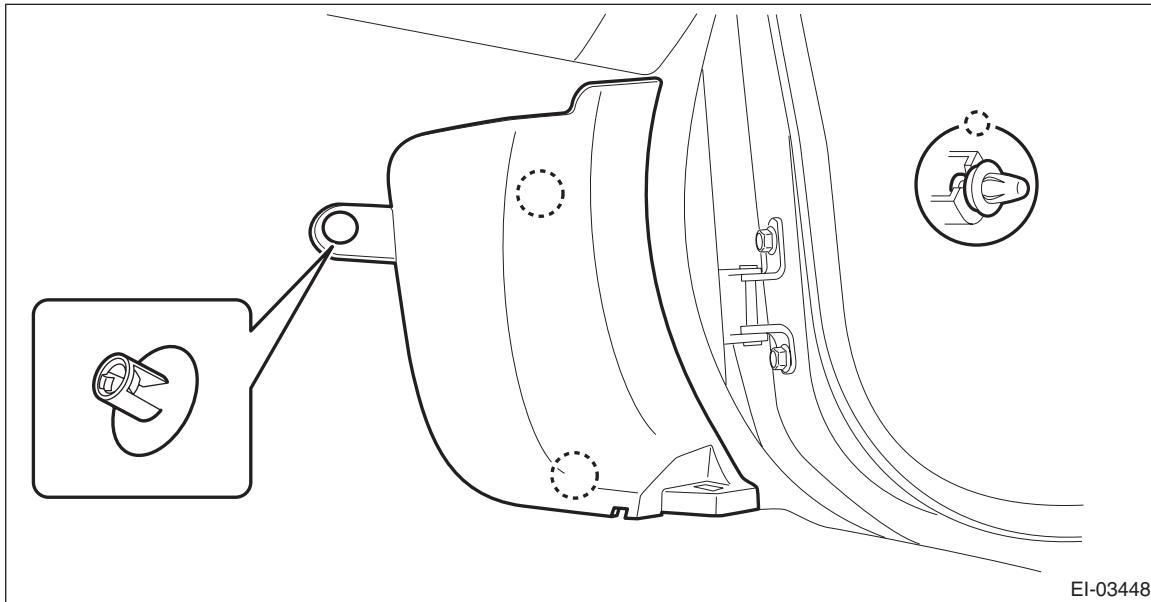
16) Disconnect the front door impact sensor harness connector. <Ref. to AB-28, FRONT DOOR IMPACT SENSOR (BETWEEN AIRBAG REAR HARNESS AND DOOR HARNESS), PROCEDURE, Airbag Connector. >
