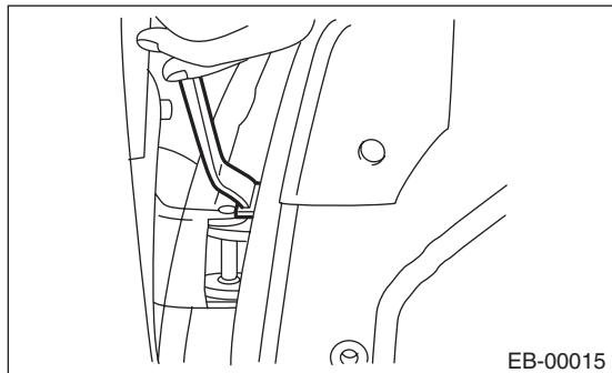
4) Remove the hinge - front door from the vehicle.
