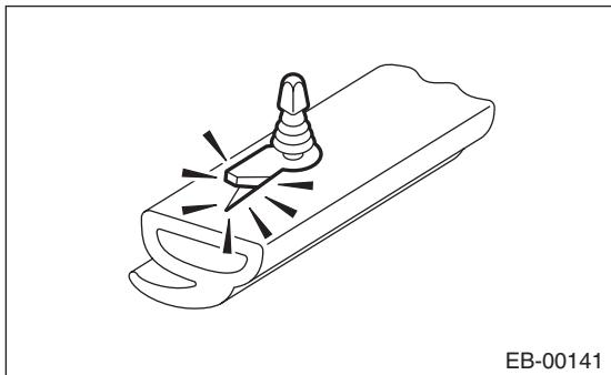
13) Remove the bolts and nuts, and then detach the checker assembly - front door.
