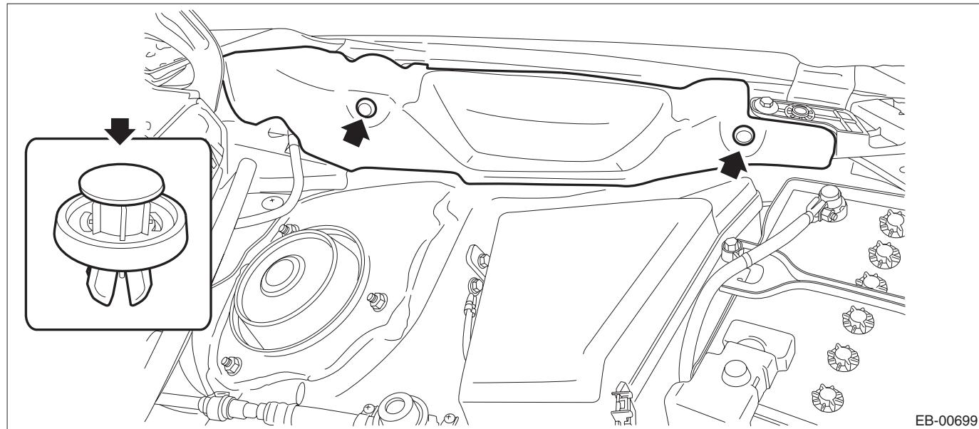
(3) Remove the light assembly - head. <Ref. to LI-27, WHEN REMOVING RH SIDE, REMOVAL, Head-light Assembly.>
