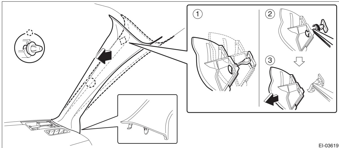
2) Release the claws, and then remove the cover side sill - front INN.
