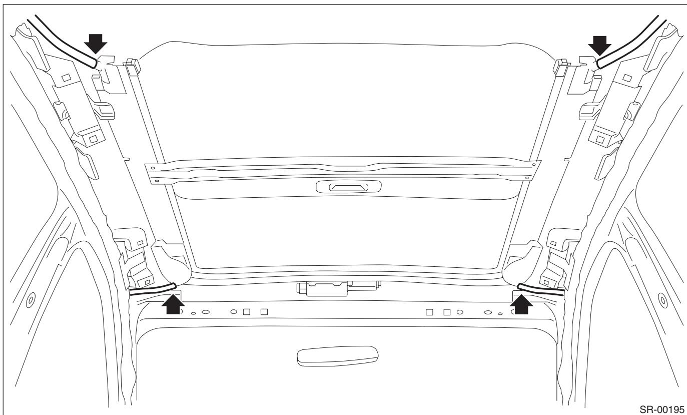
(2) Remove the bracket - assist rail.
