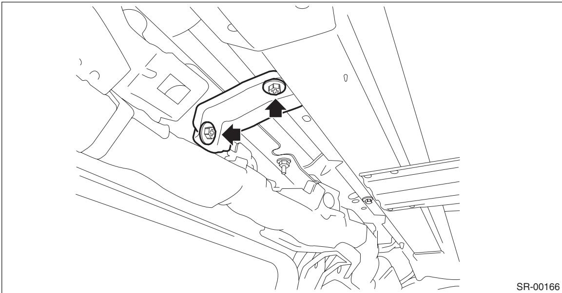
(4) Remove the bolts, then remove the rail assembly.
