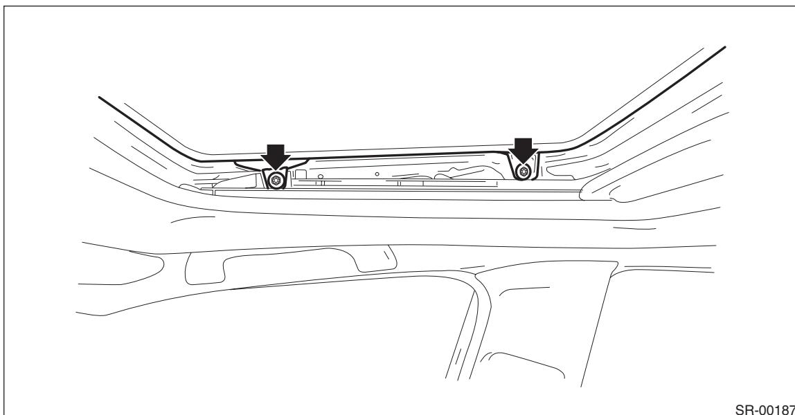
2) Remove the trim panel - roof assembly. <Ref. to EI-121, REMOVAL, Roof Trim.>
