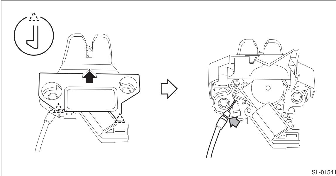
7) Remove the cable clip, and remove the cable.
