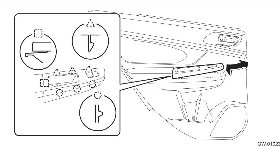
3) Release the claws, and then remove the switch - power window sub rear.
