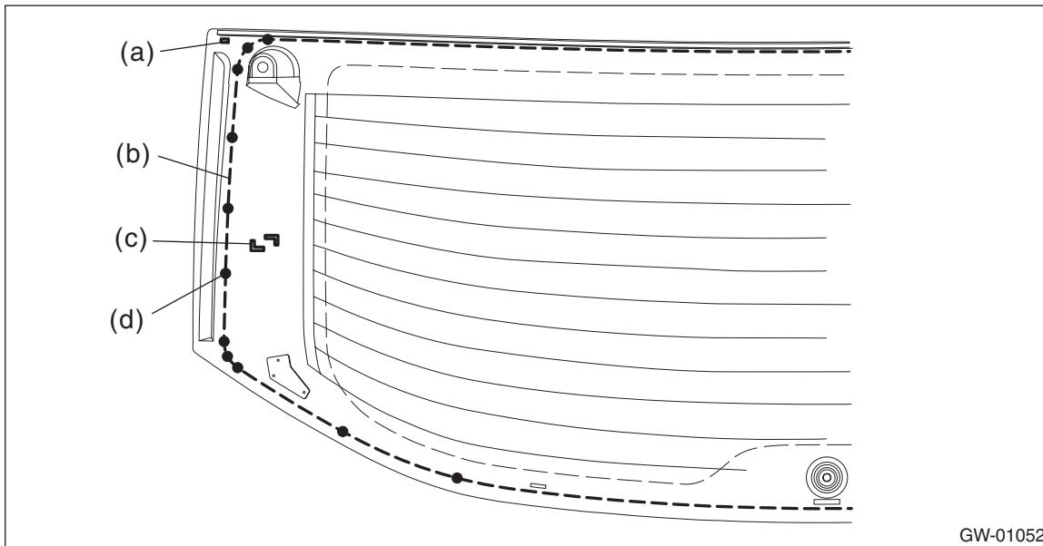
(a) Marking for dam rubber - rear gate application (Ag print)      (c) Marking for spacer - rear gate application (Ag print)      (d) Marking for primer application
