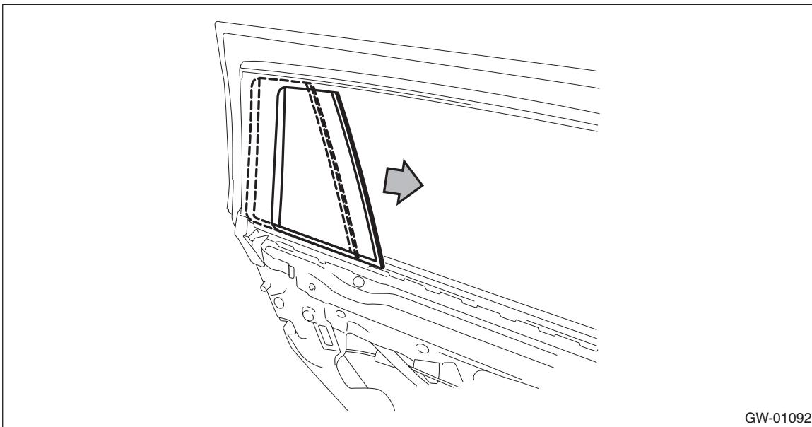
(4) While tilting the glass assembly - rear door, remove the guide from the roller of the regulator and motor assembly - rear, then remove the glass assembly - rear door.
