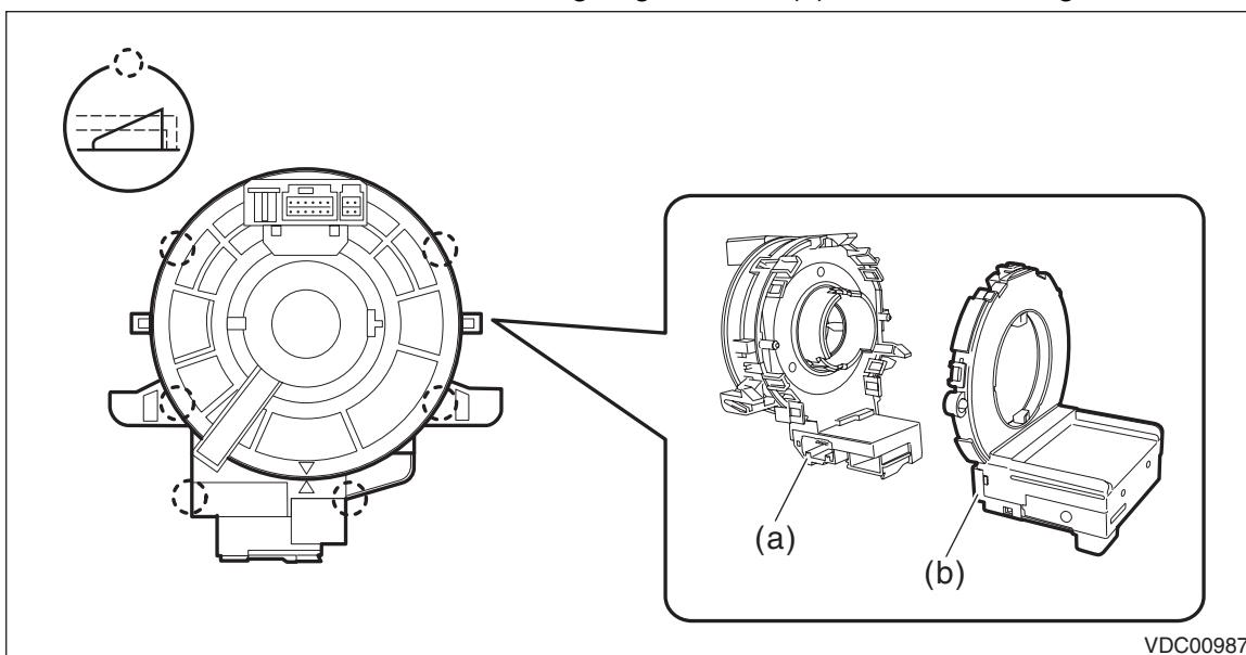
9) Install the steering angle sensor.
