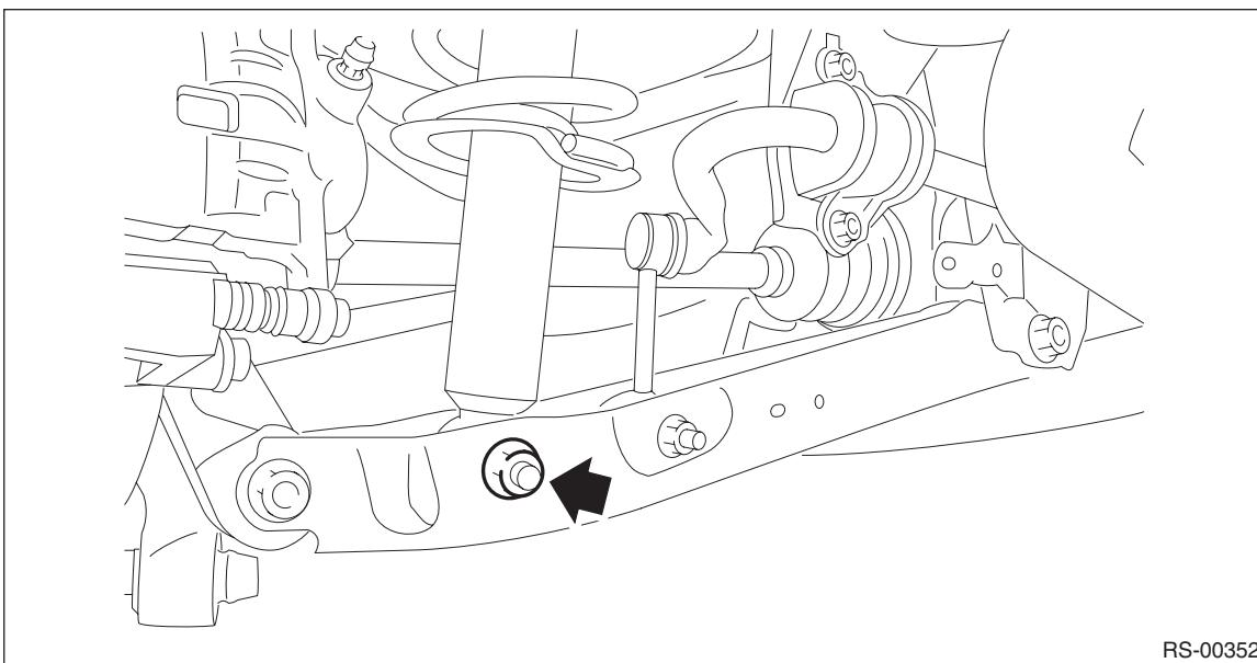
(2) Support the rear sub frame assembly using a transmission jack.
