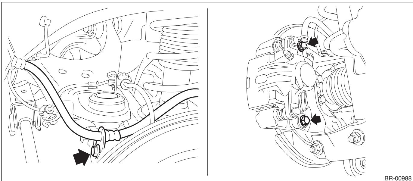
(2) Prepare wiring harnesses etc. to be discarded, and suspend the caliper body assembly from the strut assembly.
