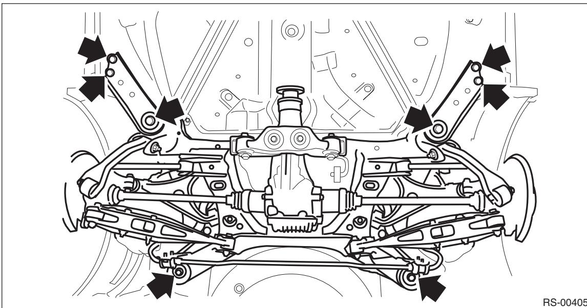
10) As necessary, remove each part from the rear sub frame assembly.
