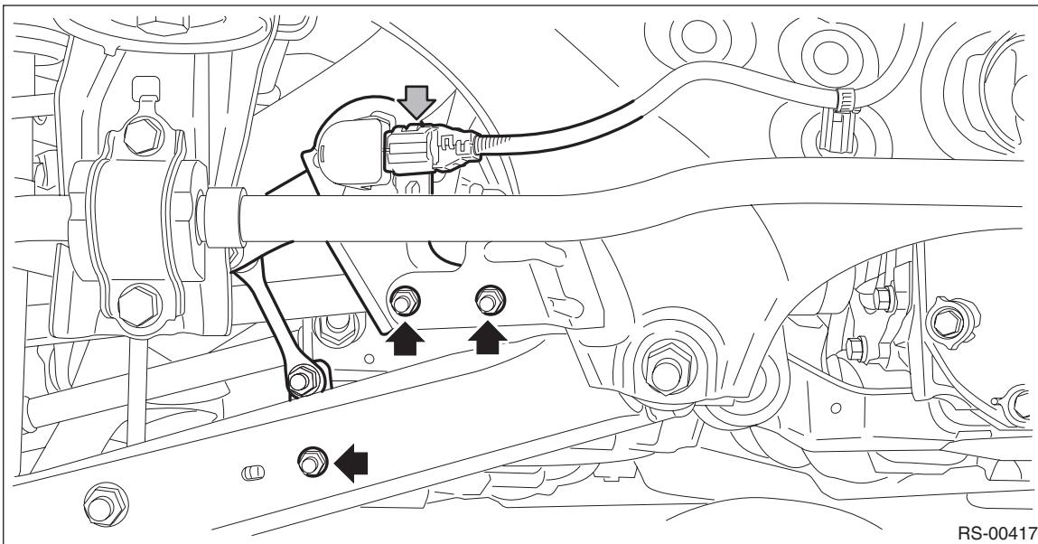
8) Remove the bolt and nuts and remove the fuel tank protector.
