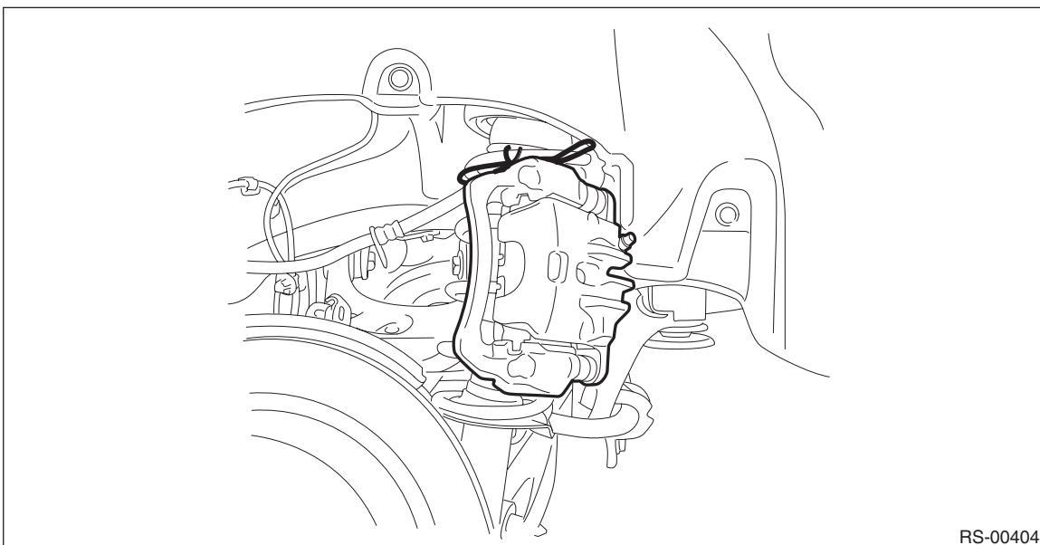
6) Remove the rear parking brake cable from the parking brake assembly. <Ref. to PB-15, REMOVAL, Parking Brake Assembly (Rear Disc Brake).>
