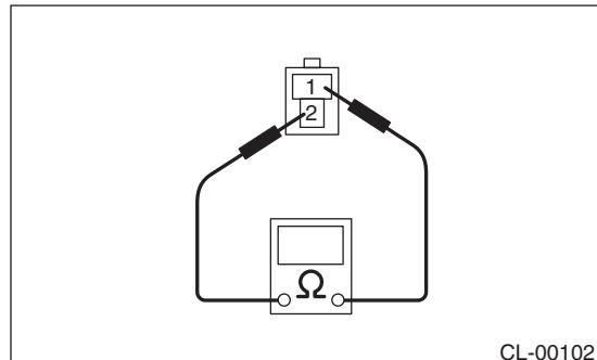
(3) Check that the switch is turned on and off in Dimension L.
