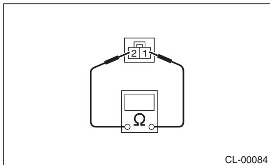
(3) Check that the switch changes between ON/OFF within L dimension.
