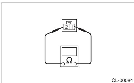
2) If the operation is not normal even when the clutch stroke and its installing condition is normal, check the continuity of the clutch switch.
