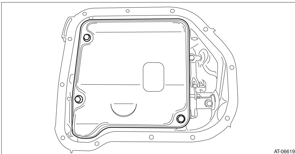
7) Remove the O-ring from oil strainer.
