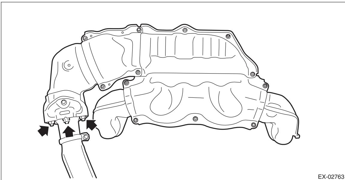
10) Remove the front oxygen (A/F) sensor and rear oxygen sensor from front exhaust pipe. <Ref. to FU(H4DO)-94, REMOVAL, Front Oxygen (A/F) Sensor.> <Ref. to FU(H4DO)-98, REMOVAL, Rear Oxygen Sensor.>
