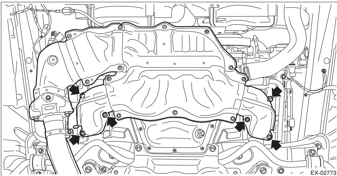
8) Remove the front exhaust pipe and center exhaust pipe from vehicle as a unit.
