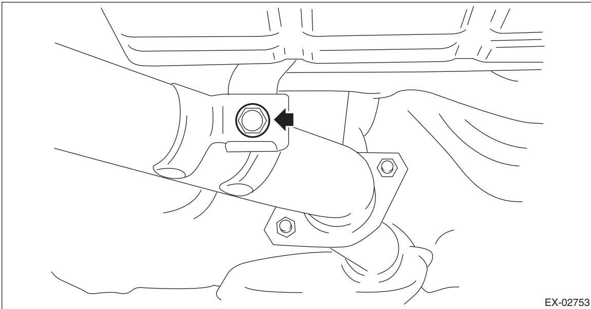
6) Remove the rear exhaust pipe from center exhaust pipe.
