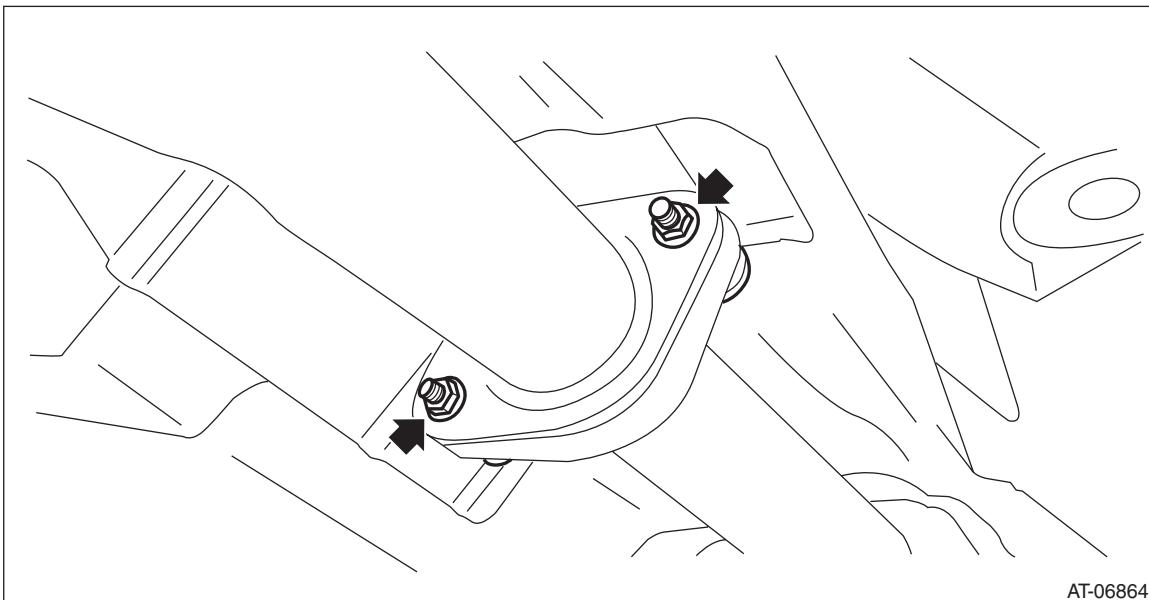
6) Tighten the bolts which secure the center exhaust pipe to the hanger bracket.
