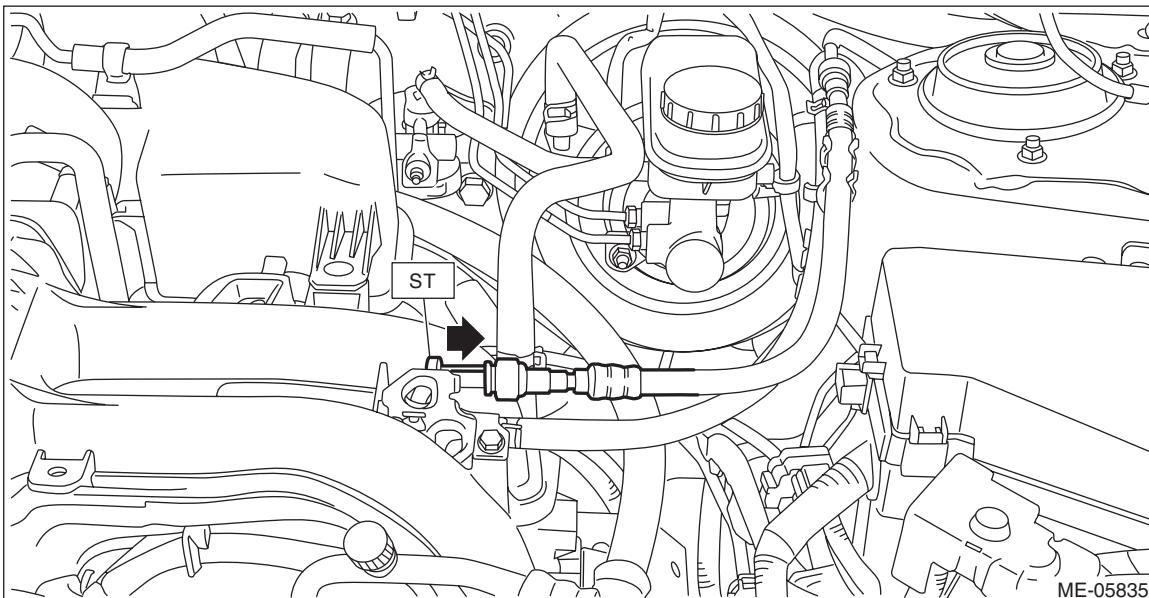
(2) Connect the fuel pressure gauge with ST1 and ST2.
