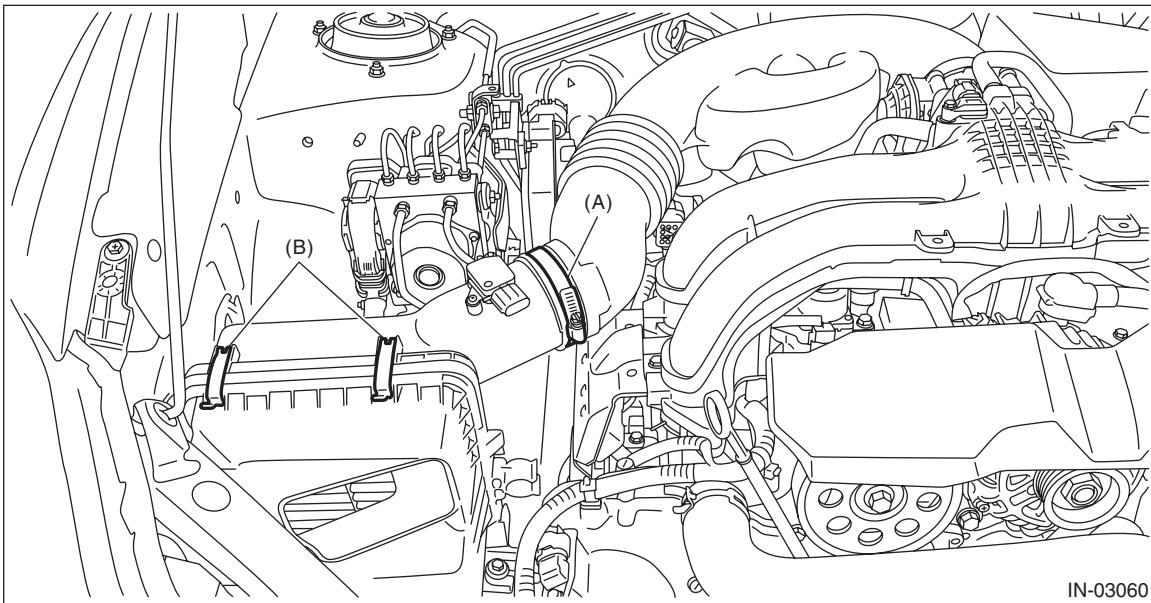
5) Remove the air cleaner case (rear) and air cleaner element.
