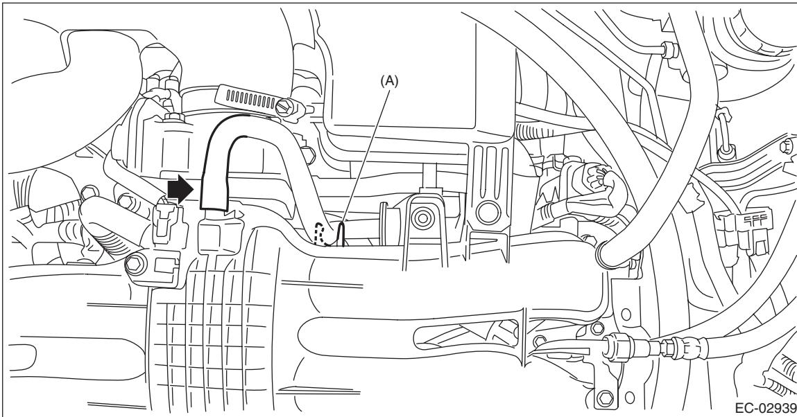
4) Disconnect the vacuum hose (A) and connector (B) from the purge control solenoid valve, and remove the purge control solenoid valve.
