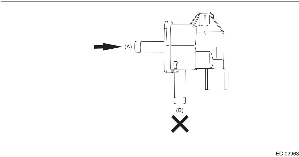
4) Connect the battery positive terminal to the terminal No. 1 and the battery negative terminal to the terminal No. 2. Check that air is discharged from (B), when supplying air to (A).
