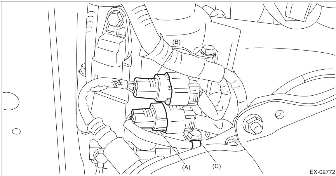
(A) Front oxygen (A/F) sensor connector
