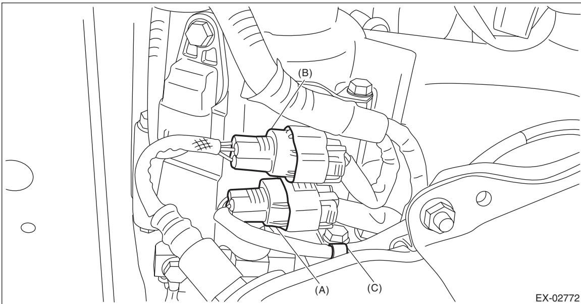
(A) Front oxygen (A/F) sensor connector
