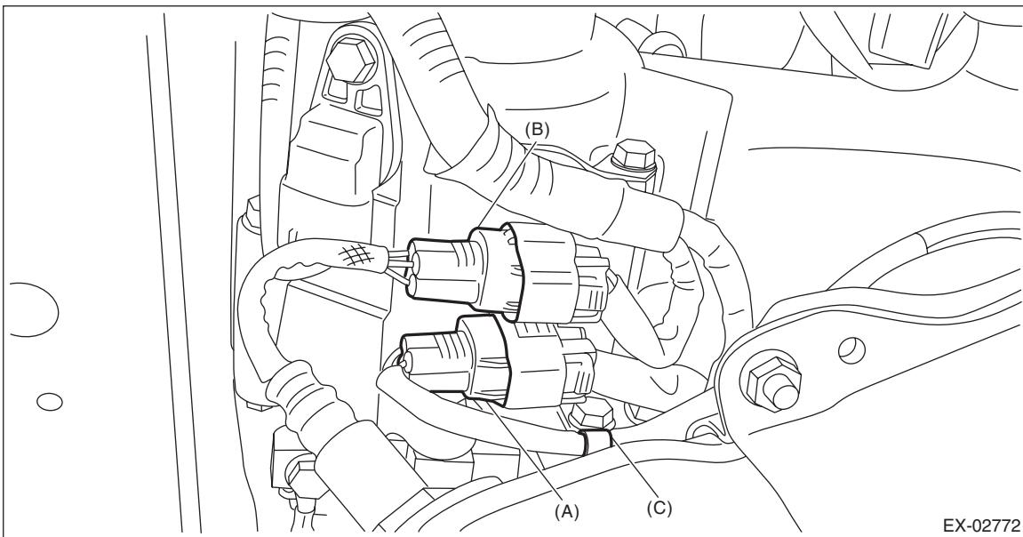
(A) Front oxygen (A/F) sensor connector
