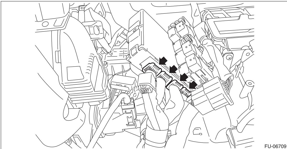
4) Remove the harness clip, and push the tabs to remove the relay block.
