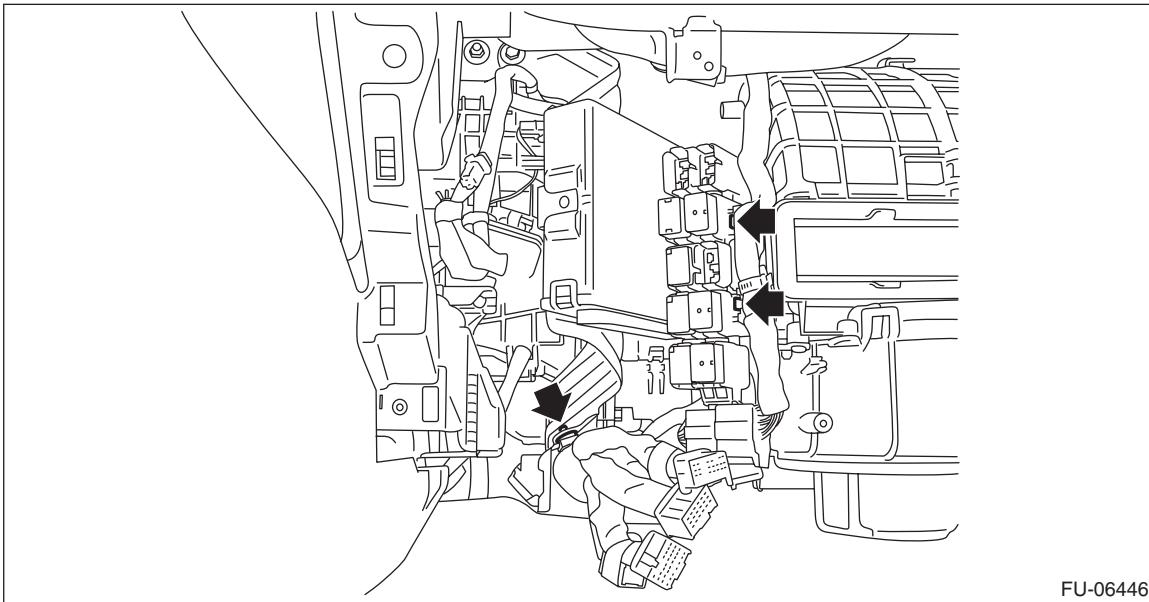
5) Remove the bolts and nuts, and remove the ECM.
