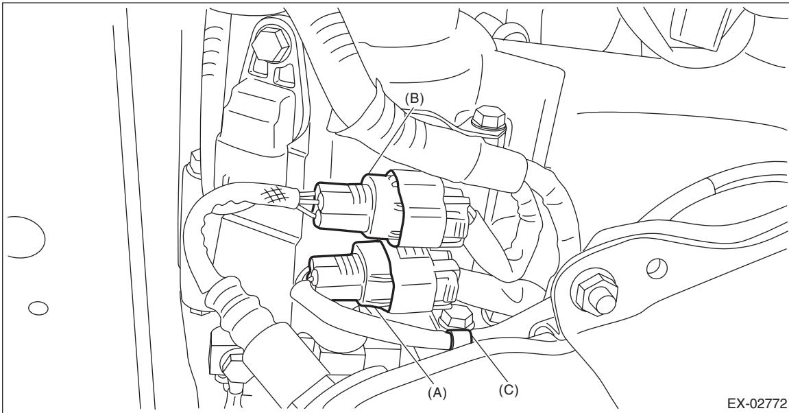
(A) Front oxygen (A/F) sensor connector
