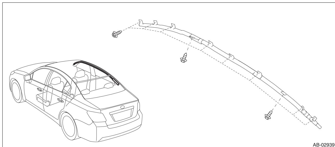
(2) Disconnect the curtain airbag module connector. <Ref. to AB-24, DRIVER'S AIRBAG MODULE, CURTAIN AIRBAG MODULE & PRETENSIONER, PROCEDURE, Airbag Connector.>
