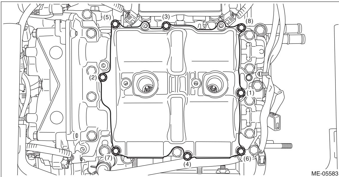
6) Install the intake manifold protector LH.
