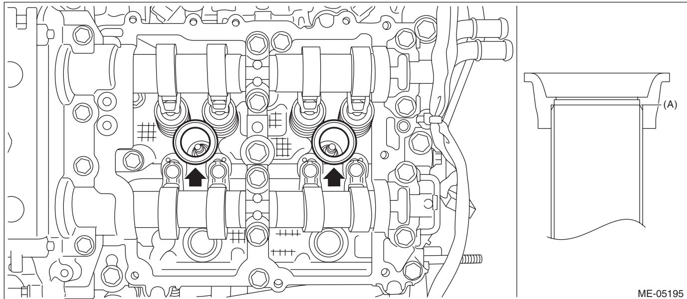
3) Install the rocker cover gasket LH to the rocker cover LH.
