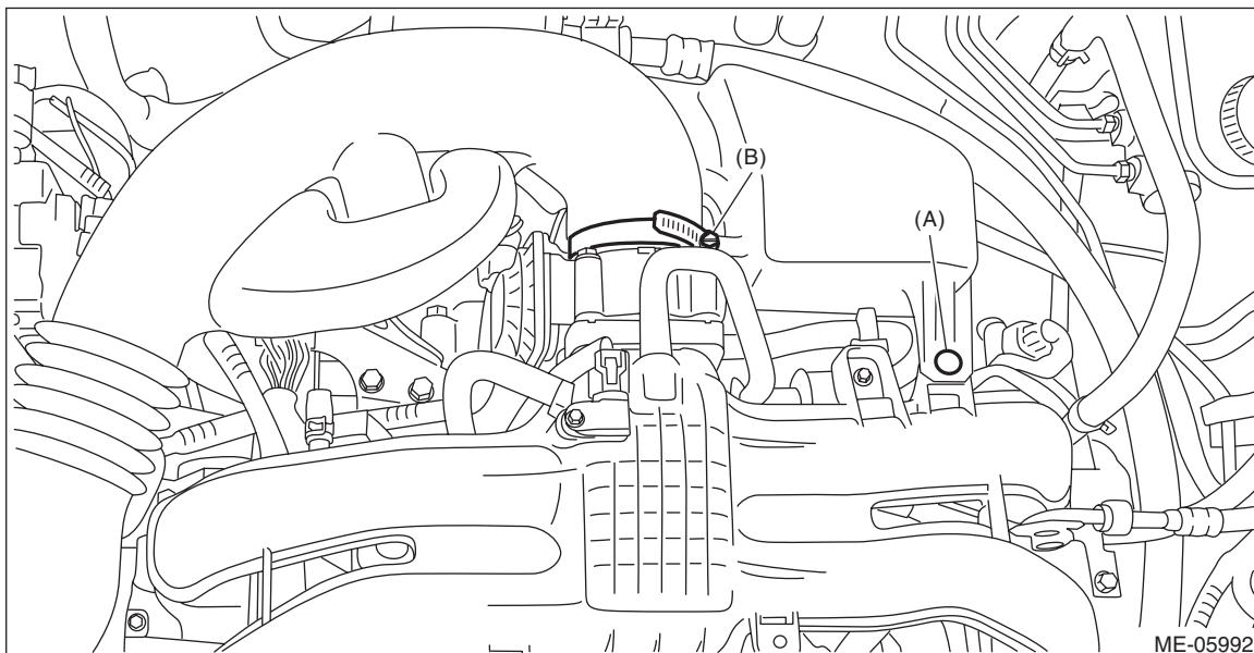
(3) Remove the air intake boot from the throttle body, and move the air intake boot to the left side wheel apron.
