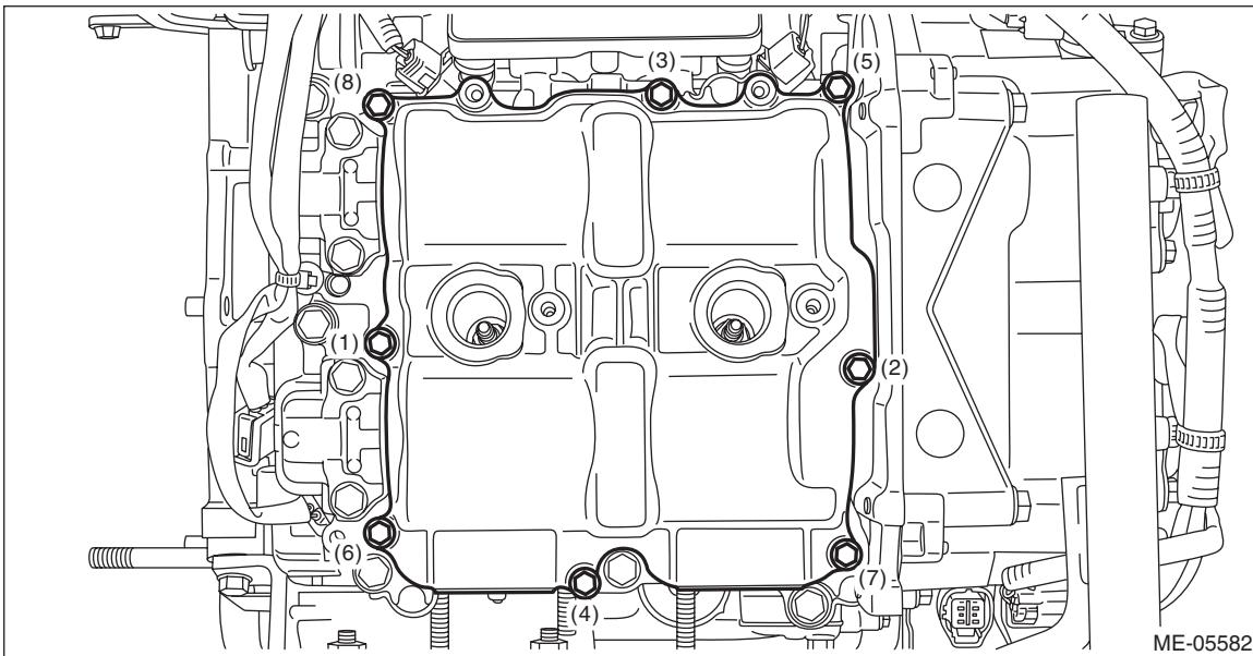
5) Install the intake manifold protector RH.
