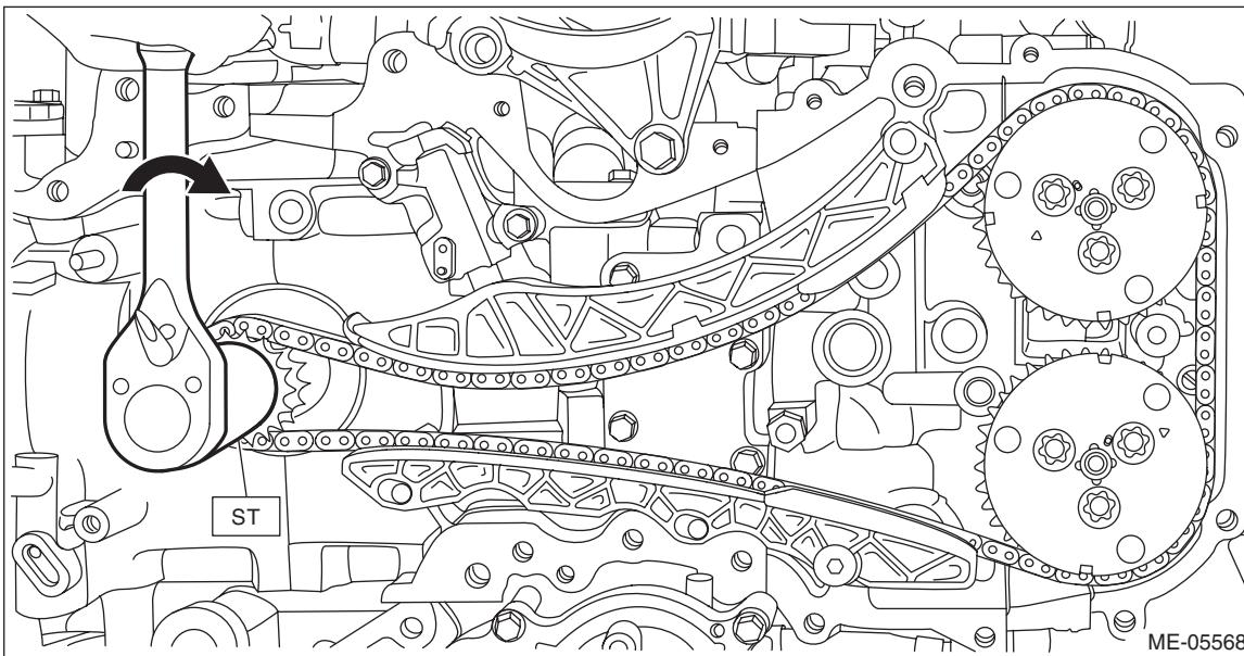
11) Install the timing chain RH. <Ref. to ME(H4DO)-121, TIMING CHAIN RH, INSTALLATION, Timing Chain Assembly.>
