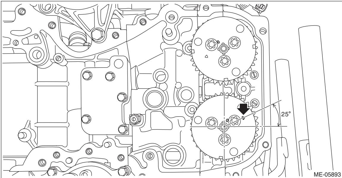
6) Install the timing chain LH and the timing chain guide LH.
