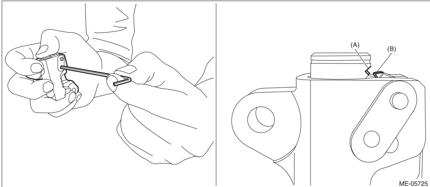
2) Check that the crank sprocket is located at the position shown in the figure. If not aligned, using ST turn the crankshaft to align the crank sprocket alignment mark to the position shown in the figure.
