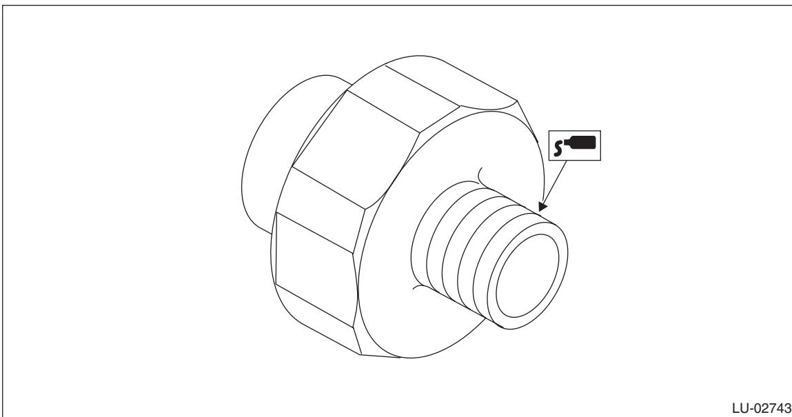
2) Install the oil pressure switch to cylinder block.
