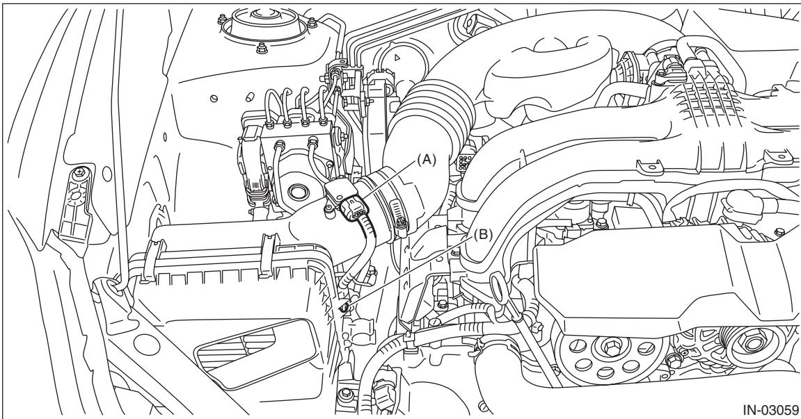
5) Install the air intake duct. <Ref. to IN(H4DO)-13, INSTALLATION, Air Intake Duct.>
