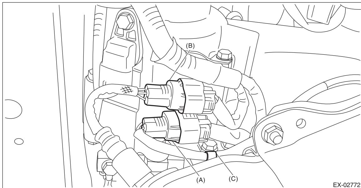
(A) Front oxygen (A/F) sensor connector
