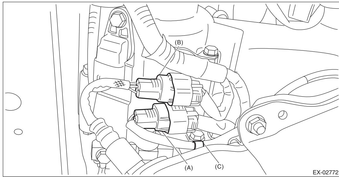
(A) Front oxygen (A/F) sensor connector
