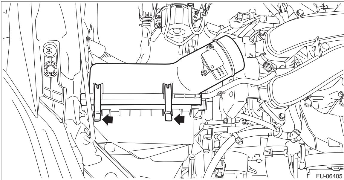
10) Remove the intake manifold protector.
