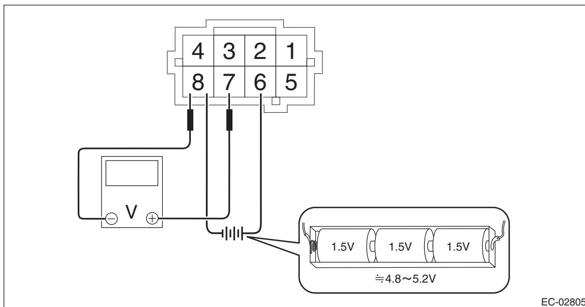
2) Check the voltage at a normal atmospheric pressure.
