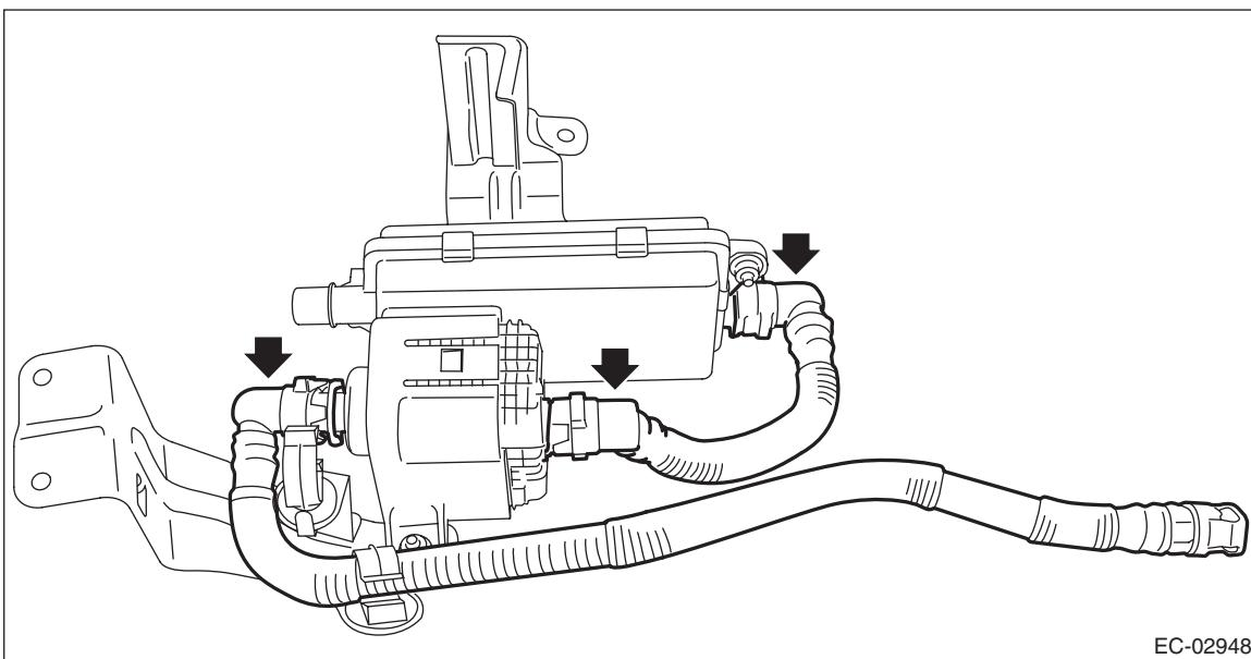
3) Install the drain separator to the leak check valve assembly. <Ref. to EC(H4DO)-53, INSTALLATION, Drain Separator.>
