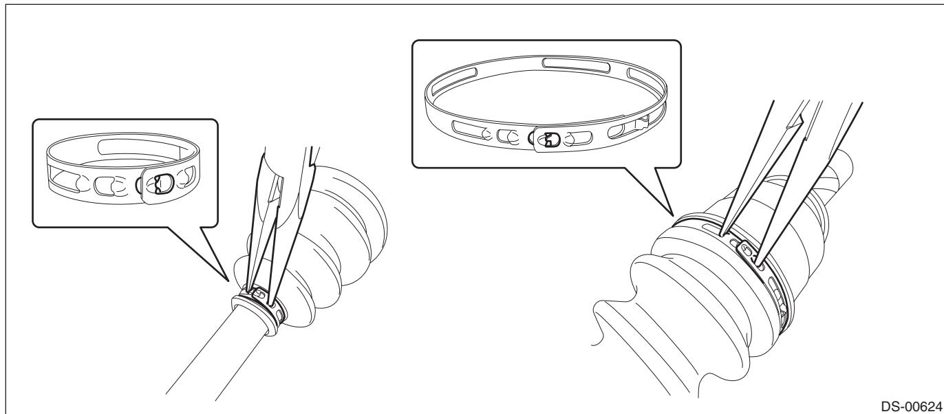
(7) Check the positions of the boot and band, align the concave claw (b) with the convex claw (d), and tighten the band.
