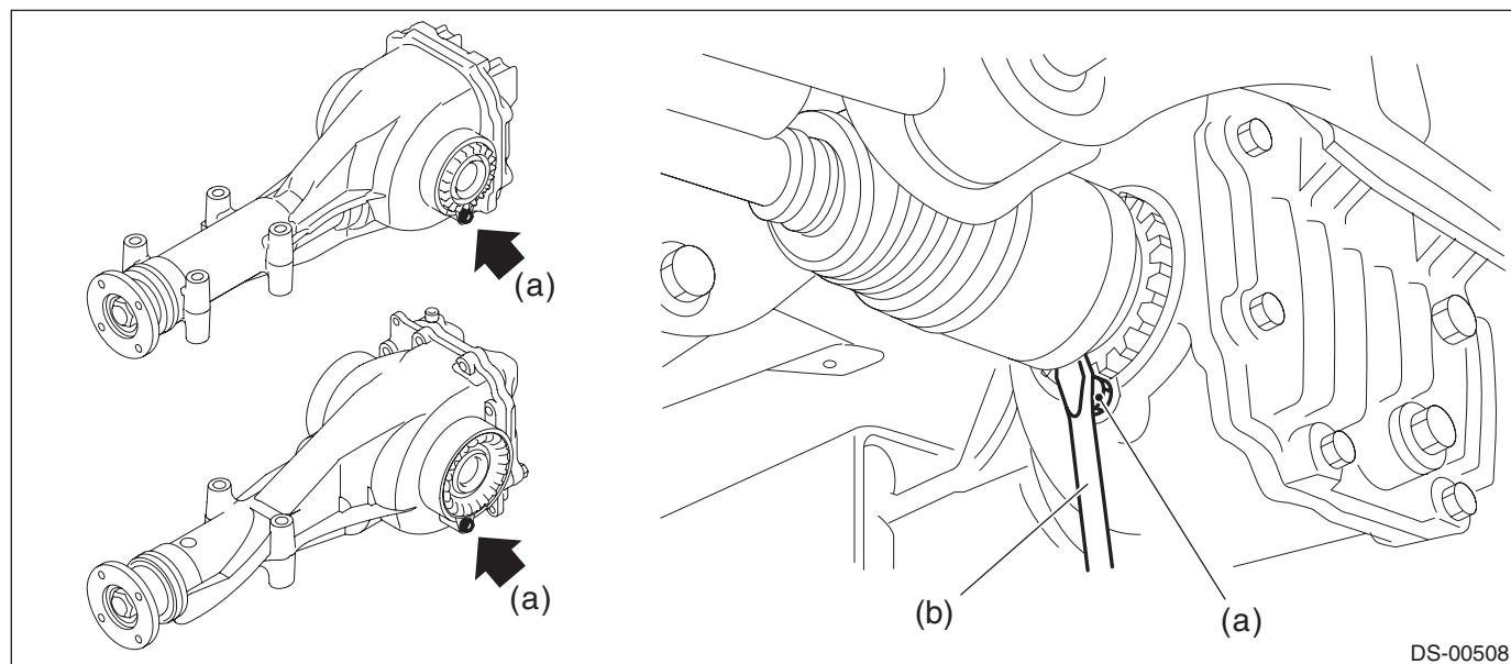
8) Remove the installation section of rear differential assembly.
