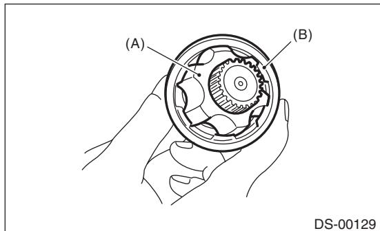
(2) Fill 80 to 90 g (2.82 to 3.17 oz) of specified grease into the inner side of the DOJ outer race.
