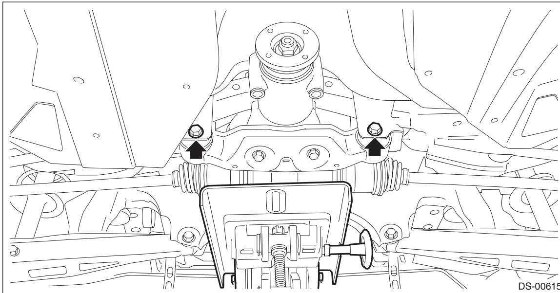
(3) Remove the self-locking nuts which hold the rear differential to the rear sub frame assembly.
