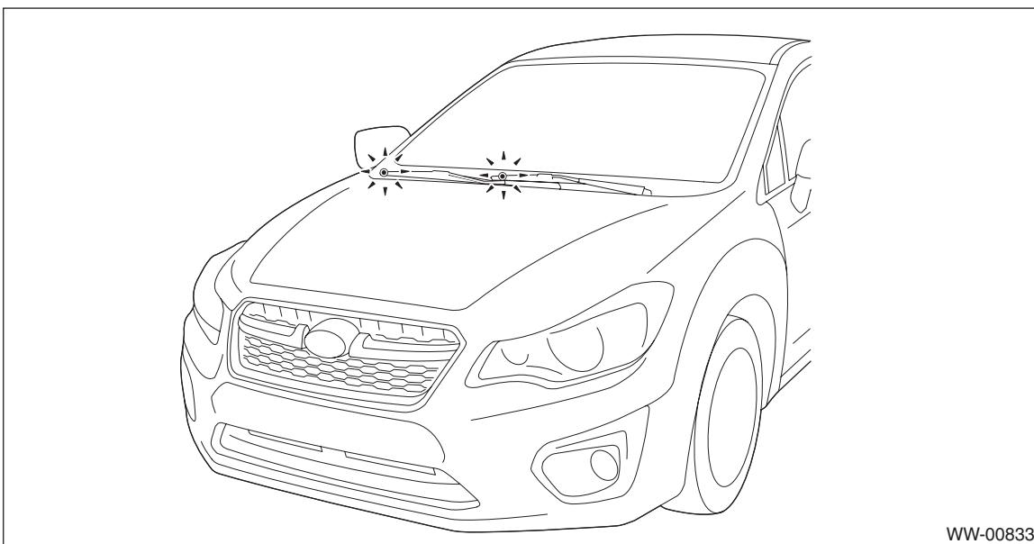
(2) Tighten the arm assembly - windshield wiper to specified torque and install the cap.
