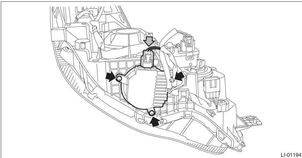
(3) Guiding the bulb socket through the gap between housing and reflector, pull out the ballast - headlight.
