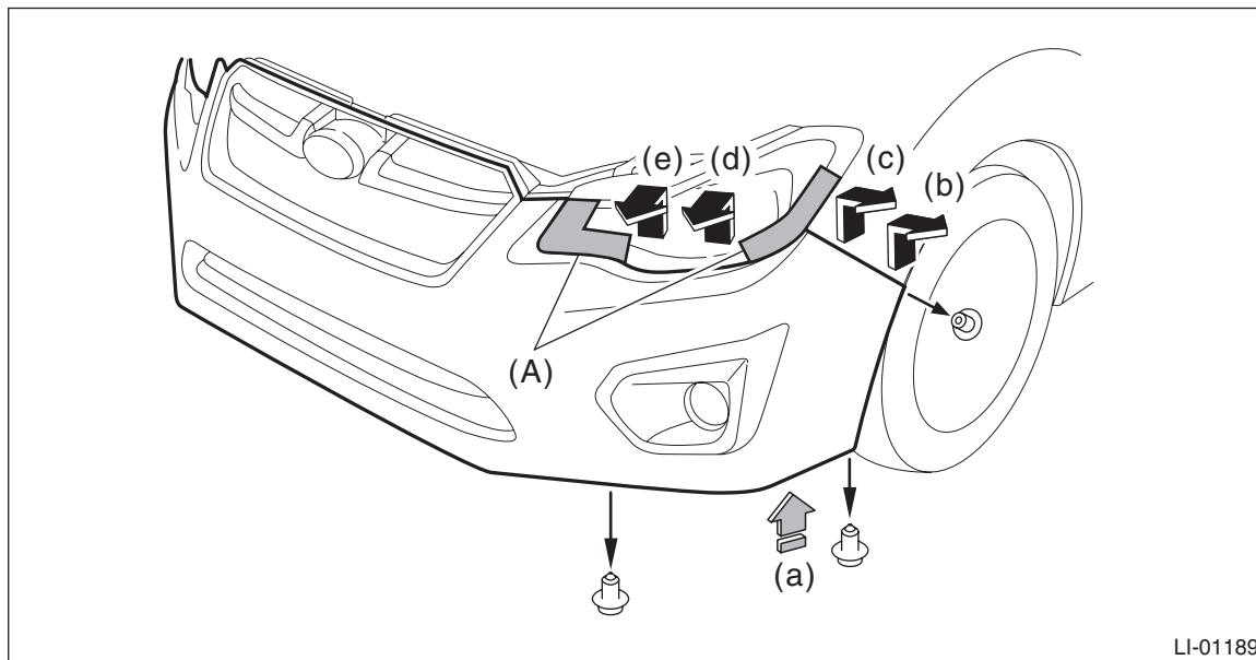
3) Remove the light assembly - head.
