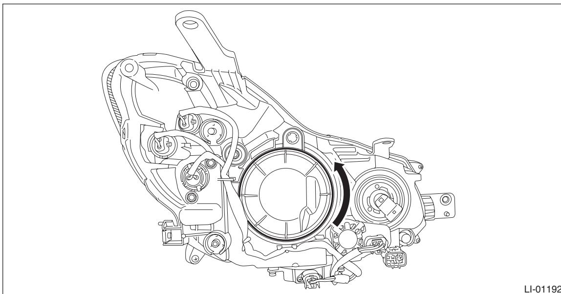
4) Disconnect the bulb socket.
