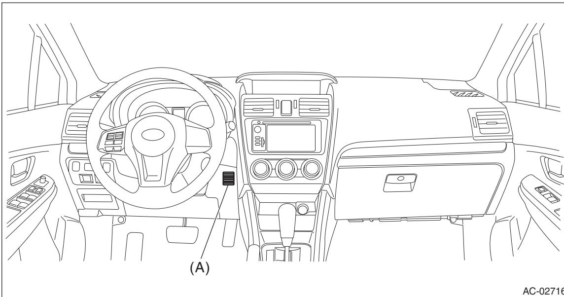
(1) Put a strip of paper close to the front side of suction port (A).
