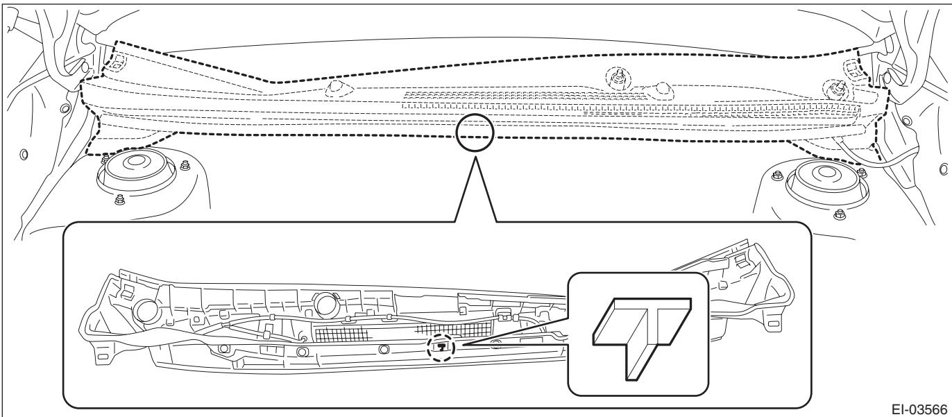
2) Install the arm assembly - windshield wiper.
