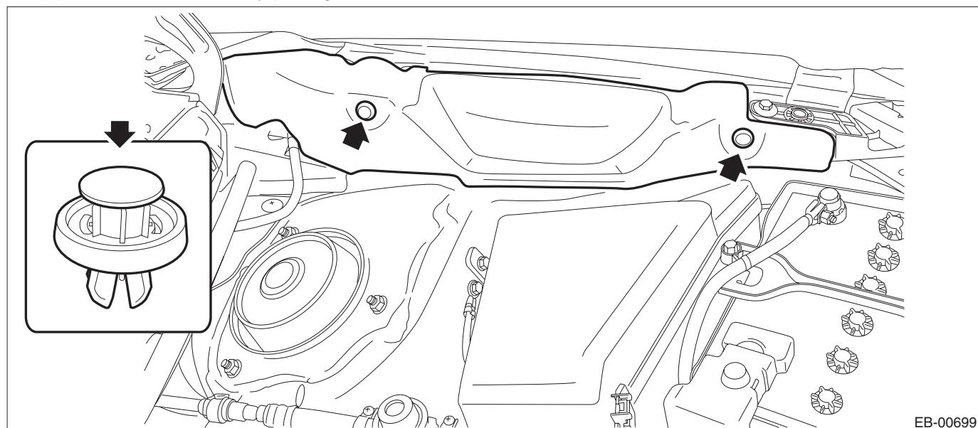
(3) Remove the light assembly - head. <Ref. to LI-28, WHEN REMOVING RH SIDE, REMOVAL, Head-light Assembly.>
