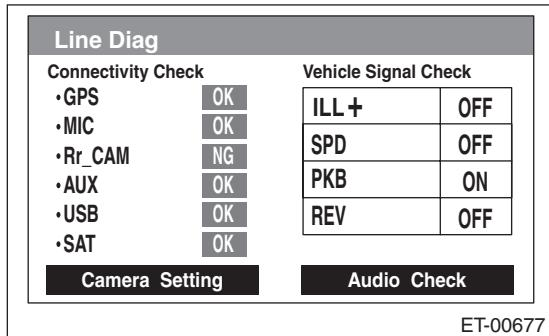
OK: Each connection device is connected correctly.
