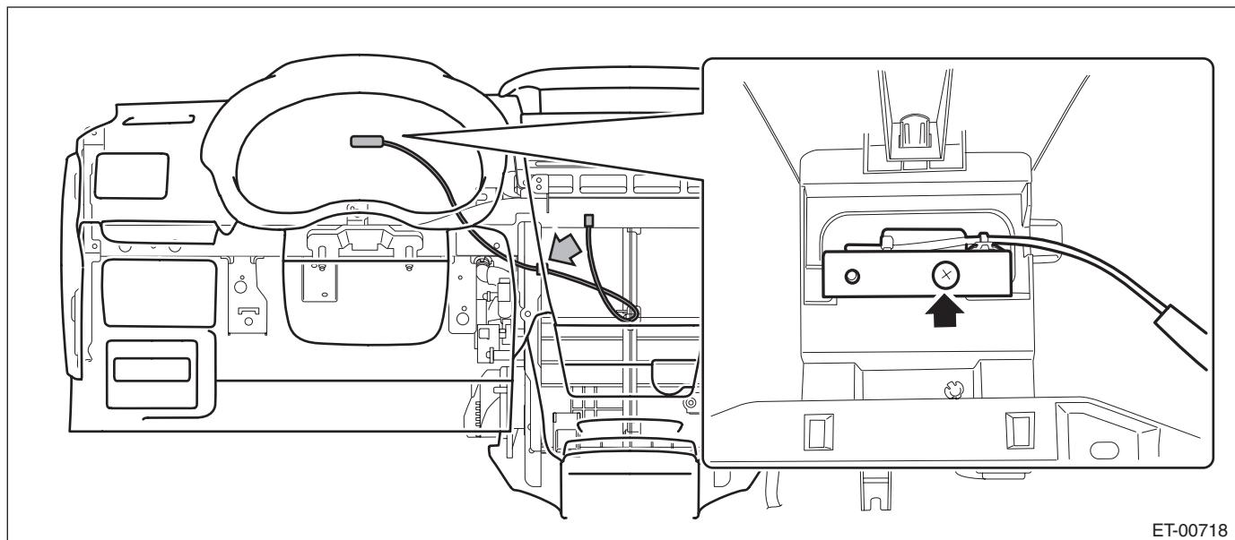
(3) When the GPS antenna assembly is pulled out, remove the string attached to the connector in step (1).
