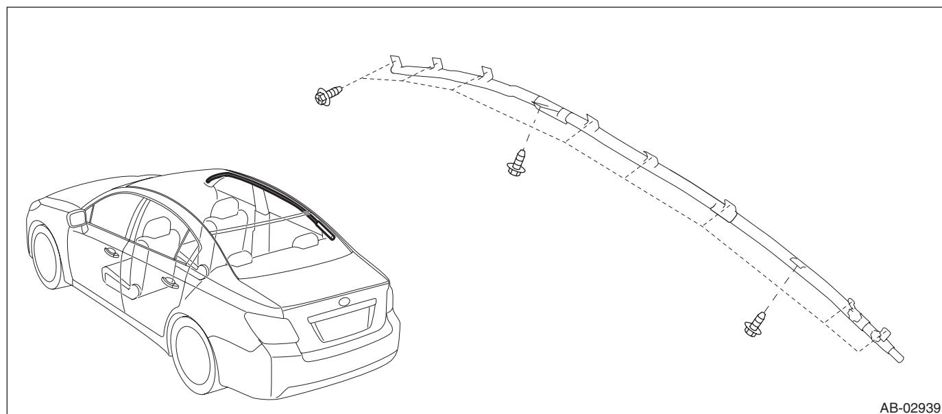
(2) Disconnect the curtain airbag module connector. <Ref. to AB-22, DRIVER'S AIRBAG MODULE, CURTAIN AIRBAG MODULE & PRETENSIONER, PROCEDURE, Airbag Connector.>
