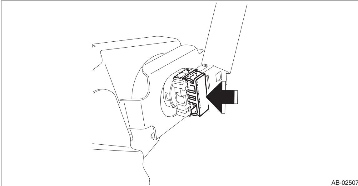
Connect the connector in the reverse order of disconnecting. At this time, be sure to insert until a clicking sound is heard.
