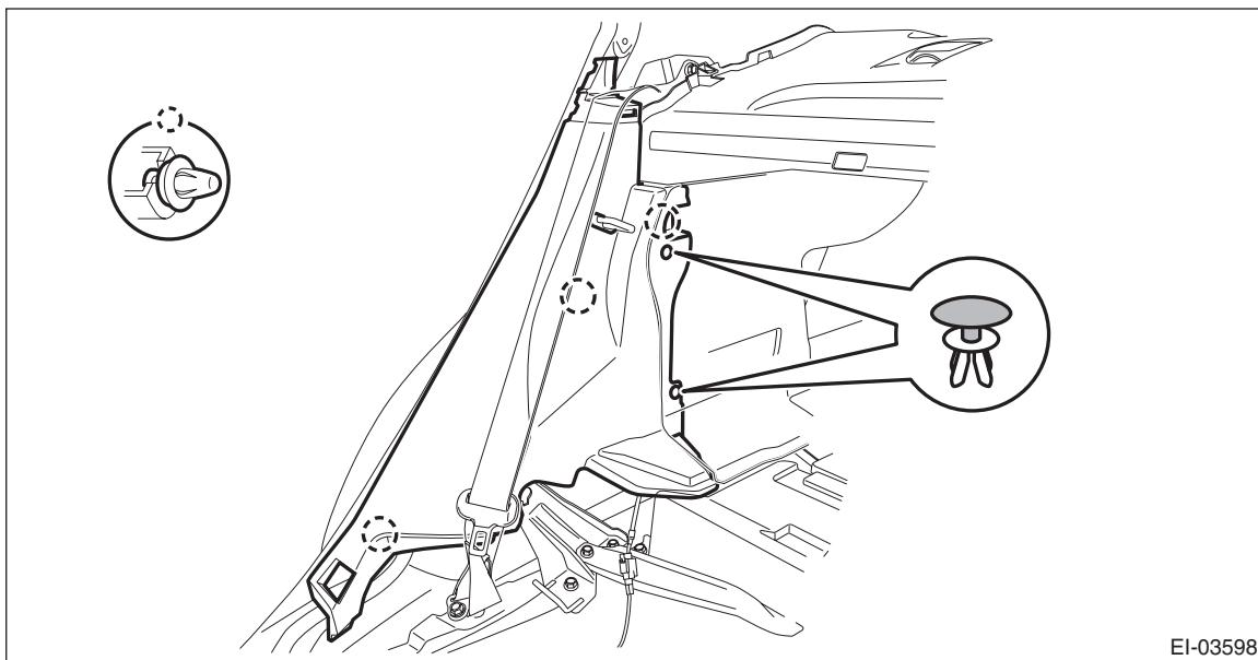
5) Remove the nuts and then remove the curtain airbag sensor. <Ref. to AB-27, SIDE AIRBAG SENSOR AND CURTAIN AIRBAG SENSOR, PROCEDURE, Airbag Connector.>
