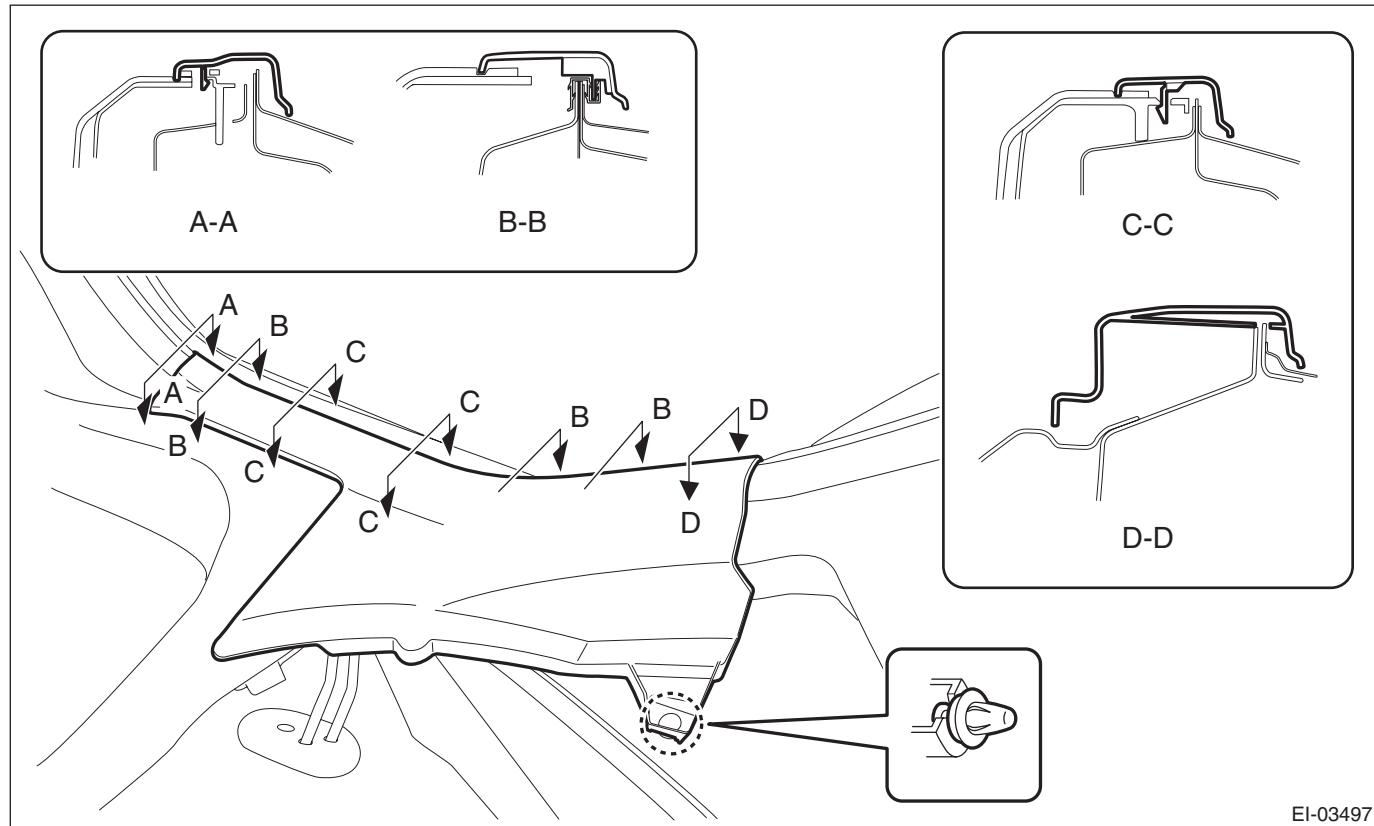
5) Remove the mat - rear floor CTR and the spacer - rear floor side.
