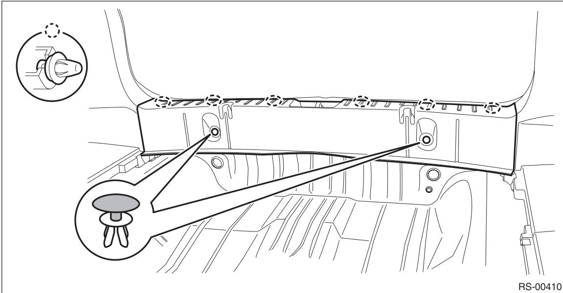
7) Remove the trim panel - rear apron. (On the side where the curtain airbag sensor is removed)
