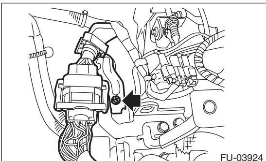
4) Slide the bulkhead harness connector in the direction of the arrow and remove it from the rear engine hanger.
