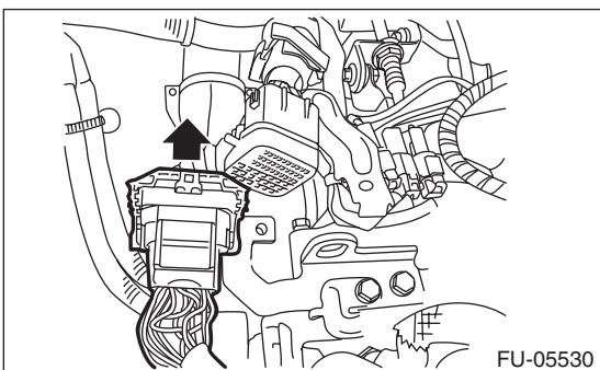
5) Disconnect the connector from the oil switching solenoid valve.
