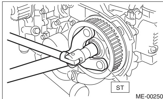
ST 499207400 CAM SPROCKET WRENCH
