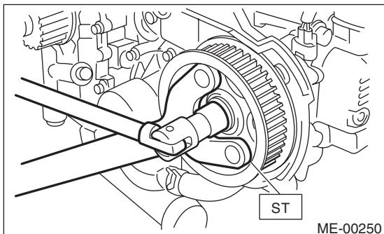
ST 499207400 CAM SPROCKET WRENCH
