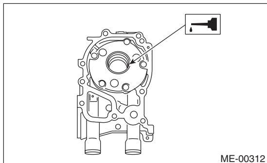
4) Install the oil pump to cylinder block.
