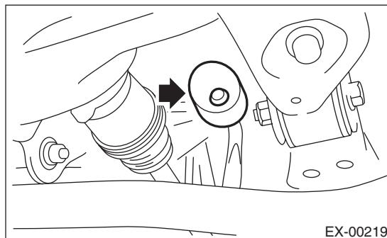
3) Install the rear exhaust pipe to the muffler.
