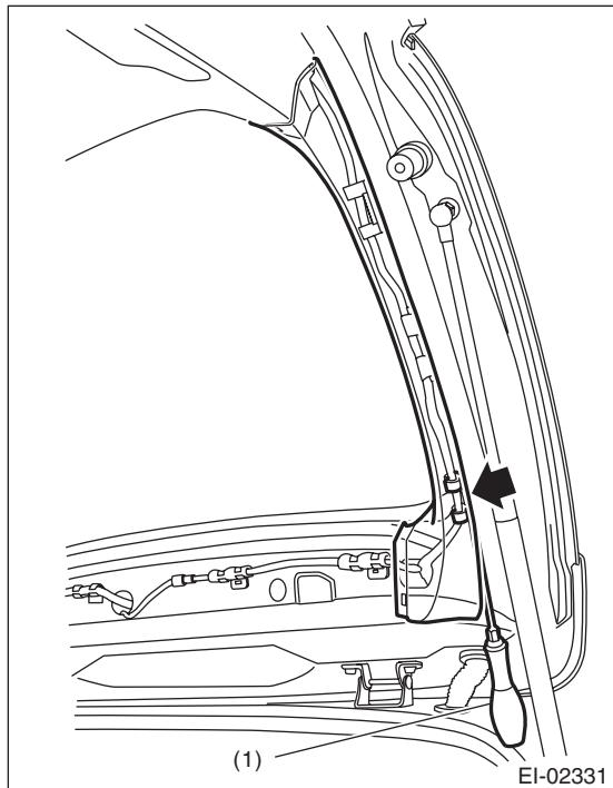
3) Remove the clips, and then remove the rear gate lower trim.
